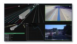
Cloverleaf turn and higher elevation reduces view of sensors
